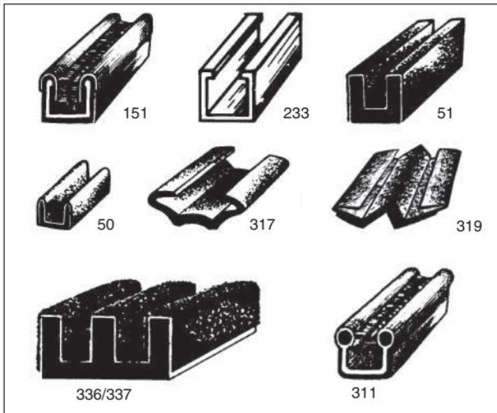
151 **Window Channel.** Single track flexible metal covered in felt/rubber. Can take 4.7mm or 6mm (5/16" or 1/4") glass. Approx. 14mm (19/16") overall width. This channel will hold its shape when bent. Can be coiled for posting ..... Per mtr
