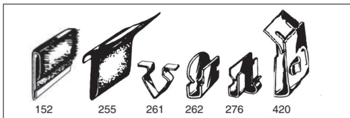
255 **Window Weatherstrip.** This is the exterior waistseal in rubber with PVC vertical insert. Black velvet covering on inner face that fits against the glass. Would seal up to 11mm ( $\frac{7}{16}$ ") gap between glass and window frame, but minimum 6mm ( $\frac{1}{4}$ ) gap unless the leading edge is trimmed down. Per 1mtr (39 $\frac{1}{4}$ ) length ..... Per length
