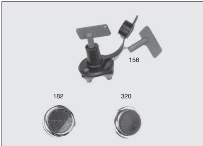
156 **Battery Master Switch.** A very basic switch with detachable red plastic key, as shown. 2 hole mounting through the body with hole centres approx. 41mm (1½"). Controls circuits of up to 300 amps at 12 or 24 volts. To switch off and isolate circuit, turn anti-clockwise and remove key ..... Each
