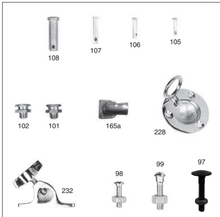
232 **Hood Fastener.** Chrome on brass. To suit 16mm ( $\frac{5}{8}$ ") dia. peg. Mounting hole centres 49mm ( $1\frac{15}{16}$ "). ..... Each
